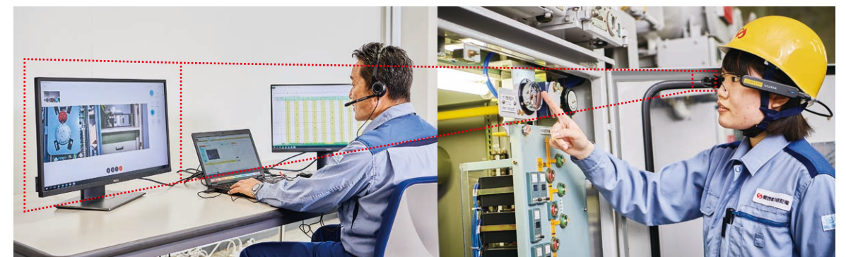
Remote support for on-site operations using smart glasses (glasses-like devices equipped with cameras and microphones)
